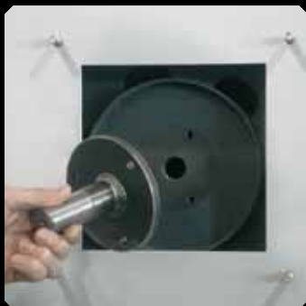
A re-lagging door on both sides of the head allows for easy removal and installation of the slide lags without breaking the belt.
