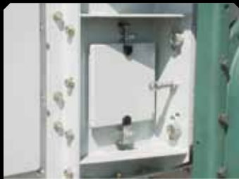
A re-lagging door on both sides of the head allows for easy removal and installation of the slide lags without breaking the belt.
